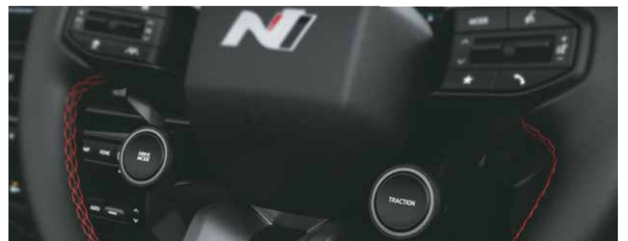
Drive mode select – Eco, Normal, Sport | Traction control modes – Sand, Mud, Snow (New)
